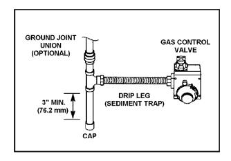
FIGURE 19. GAS PIPING WITH FLEXIBLE CONNECTOR.
